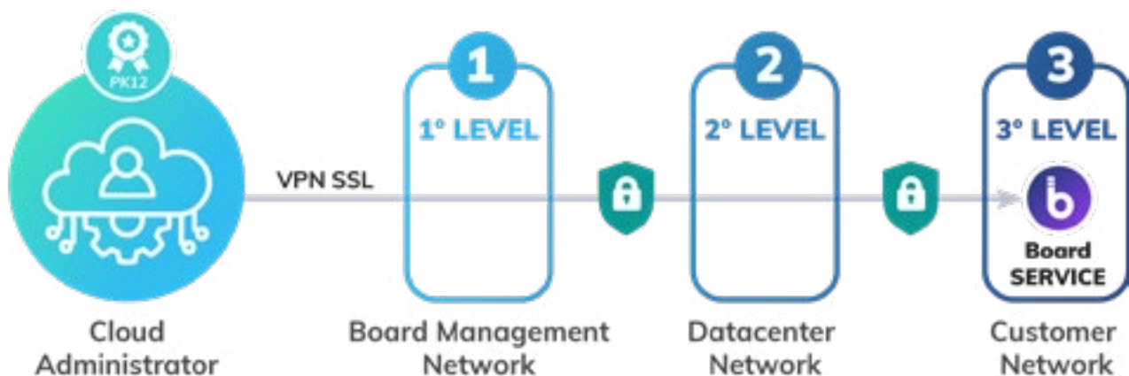
Fig. 8 – Access Restriction and Network Segregation*
